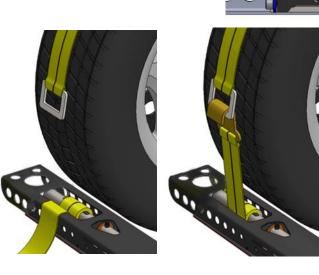
6. Use 1/2" drive ratchet to tighten winch, rotate counter-clockwise. Take up slack on both sides, then tighten two more clicks on each side.
