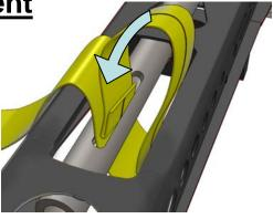
**3.** Make sure hemmed part of strap grabs inside wall of tube. If it does not, then wrap around the tube in the opposite direction.
