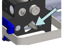
2. Unhook strap coupling and remove straps from tire.
